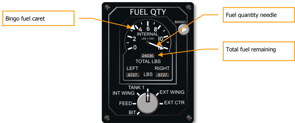
Figure 35. Fuel Quantity Indicator
