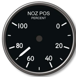
Figure 34. Engine Exhaust Nozzle Position Indicator
